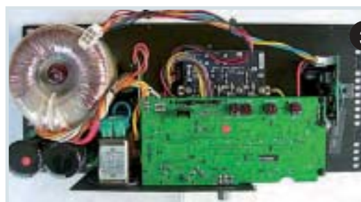
03 / Class AB for high frequencies, Class D for low frequencies.
