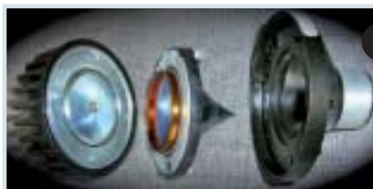
02 / Anatomy of a compression driver from EV, showing from left to right: the casing/radiator supporting the pole pieces and the neodymium magnet, the dome diaphragm and the moving coil mounted on the conical phasing plug, with a 1" throat and threaded attachment section to the horn.
