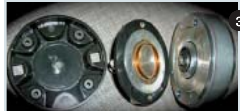
02 /Mineral wool behind the M34 compression driver 03 /Tweeter with, from left to right, rear casing, titanium diaphragm and phase plug at the heart of the ferrite magnetic unit.
